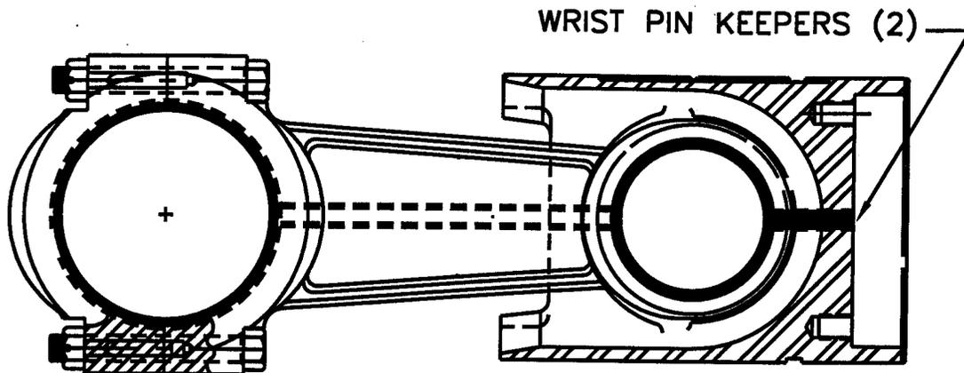
FIGURE 4-4 Crosshead Assembly
